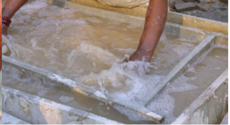
Once the lokta plants are ready to harvest, the branches will be decorticated and the bark is being watered and then beaten until they can take out the bast. In the next step the bast is shredded to fine fibres and water is added to create a nice „not too stiff, not to fluid“ pulp.
