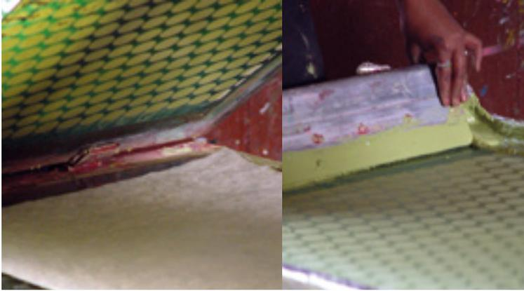
The silk screen process in Nepal is still „all handmade“, without machines. The screens are prepared and the sheets are being printed the „old fashioned way“ – without vacuum or other „helping hands“. After printing the sheets will be dried in racks and as some colours cannot be exposed to the sunlight - these are dried inside the workplace.
