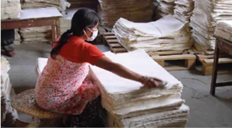
Generally the sheets are produced in the villages in the hilly regions of the Himalaya and from there the sheets arrive in the warehouses of our producers. Here they will be sorted and controlled, flattened and calendered. The calendering process is essential for the fineness and the smoothness of the sheets. They are put on metal sheets and will then „roll“ through a calendering press.
