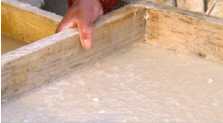
After it is evenly spread, the frame is pulled from the bassin and the water flows back into the bassin. Once the water has dripped off, the frame will stand upright in the sun until the sheet is dry.
